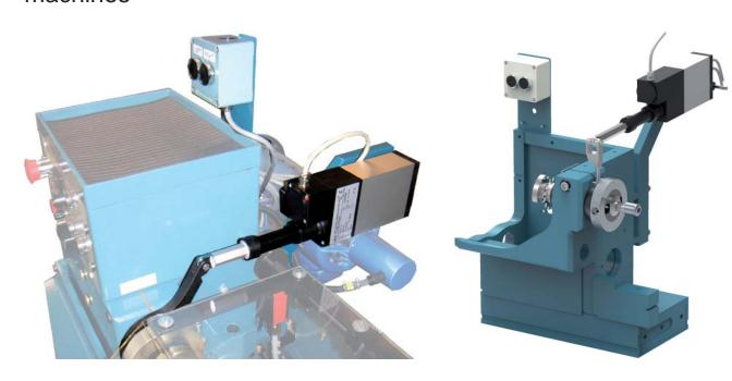
The most frequent and most important set adjustment when setting a band saw is the symmetry adjustment. The new versions of the SGS software (5.01 and later) will now allow the ALO 185 set gauge to control the set symmetry and continuously make adjustments by means of a servo motor. This will give you advantages such as less stops for operator adjustments, possibility to keep a tighter symmetry / balance tolerance on your bands, and a lower scrap percentage due to miss adjustments.
