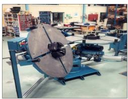
Picture showing tilt able take up coiler
