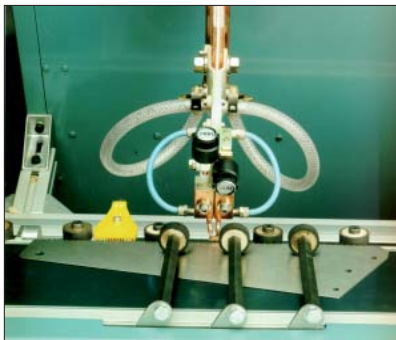
Tempering inductor and air cooling
