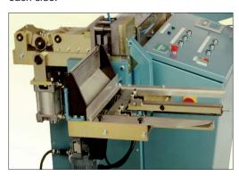
Picture showing compact toggle joint and collect magazine.
