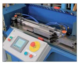
The feeding system with clamping jaws on each side.
