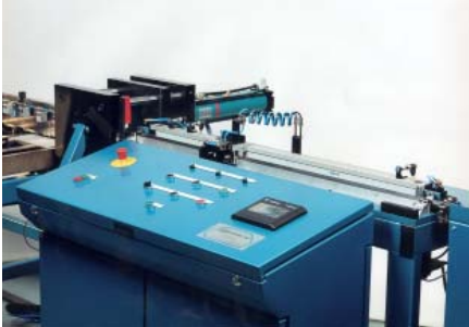
Feeding system with programmable linear feeder.
