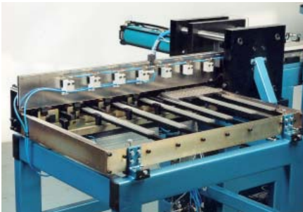
Collect magazine with pneumatic press. Blades are vertically stacked.
