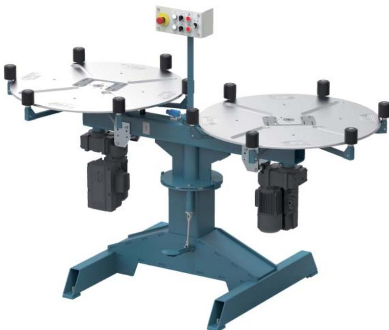
ALO 831 has a sturdy design with a welded steel frame and the plates of aluminium have machined slots to facilitate bundling and loading/un-loading of coils with hoist equipment or similar.
