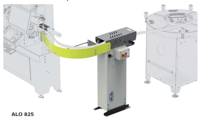
Designed to maintain an automatically controlled loop of band being fed into ALO's setting machines. The unit has a pair of pneumatically compressed feed wheels that are driven by a frequency controlled AC motor. The two wheel drive system ensures that the band have no slipping problems.
